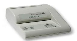
cheques to be processed every day. The bank's code number and cheque number are printed on the cheques with a special type of ink that contains particles of magnetic material that are machine readable. This reading process is called Magnetic Ink Character Recognition (MICR). The main advantage of MICR is that it is fast and less error prone.
