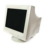
large vacuum tube, called Cathode Ray Tube (CRT). The CRT display is made up of small picture elements called pixels. The smaller the pixels, the better the image clarity, or resolution.
