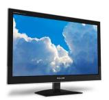
The flat-panel display refers to a class of video devices that have reduced volume, weight and power requirement in comparison to the CRT. Current uses of flat-panel displays include calculators, video games, monitors, laptop computer, graphics display.
