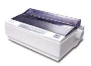
one point of time. It is a very versatile and inexpensive output device. In dot matrix printer the print head physically "hits" the paper through the ribbon and produces text (or images) by combinations of dots; hence the name dot matrix printer. Its speed is measured in **characters per second (CPS).** Although it is less expensive, it is louder, slower and produces lower
